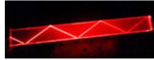
Total internal reflection between parallel surfaces enclosing dense medium: mechanism to make light travel longitudinally (fiber optics)
