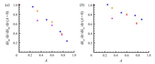
FIGURE 14. Atwood number effects on mixing layer growth rates measured by (a) momentum thickness and (b) vorticity thickness for the  $(\blacksquare)$  present incompressible INBM simulations,  $(\bullet)$  the LMNOB (thermal variation) simulations of Almagro *et al.* (2017) and  $(\blacktriangle)$  0.7 Mach number NOB (thermal variation) simulations of Pantano & Sarkar (2002). The growth rates are scaled by the corresponding growth rate with  $A \approx 0$  for each data set.
