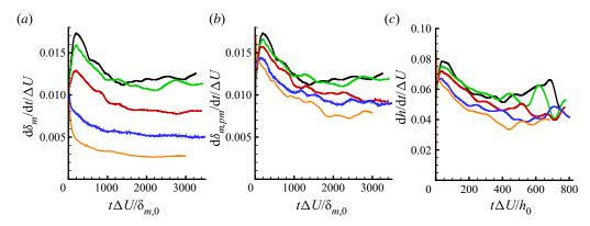
FIGURE 4. Time evolution of mixing layer thickness growth rates based on (a) momentum thickness  $\delta_m$ , (b) momentum thickness per unit mass  $\delta_{m,pm}$  and (c) mean velocity thickness h. These correspond to the time derivatives of the thickness evolutions shown in figure 3.
