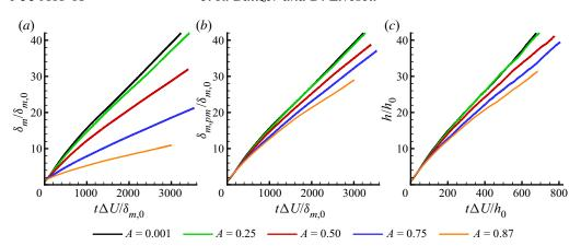
FIGURE 3. Mixing layer widths: (a) momentum thickness  $\delta_m$ , (b) momentum thickness per unit mass  $\delta_{m,pm}$  and (c) mean velocity thickness h time evolution for each Atwood number. Lines are coloured by Atwood number: A = 0.001 (black); A = 0.25 (green); A = 0.50 (red); A = 0.75 (blue); A = 0.87 (orange).
