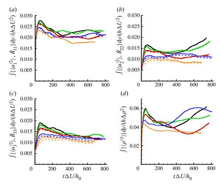
FIGURE 7. (a-c) Time histories of y-integrated planar-average turbulence intensities  $\langle u'_i u'_i \rangle$  (——) and corresponding Favre-average Reynolds stresses (- - -), each divided by Favre mean streamwise velocity thickness h for the (a) streamwise, (b) cross-stream and (c) spanwise components. (d) Time histories of y-integrated planar-average density fluctuation intensities. Line colours for each Atwood number are as for figure 3.
