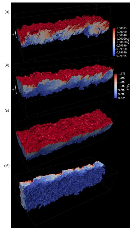
FIGURE 17. Surfaces of density coloured from light (blue) to heavy (red) during self-similar growth at approximately  $t\Delta U/h_0=730$  for (a) A=0.001 and (b-d) A=0.75. Viewing the A=0.75 case from below (d) makes apparent the much finer scales on the light fluid side relative to the heavy fluid side (c). This is consistent with the strongest turbulent vortices being concentrated near the light fluid side. Thickness h as defined based on the velocity field is also included.
