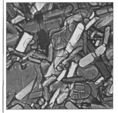
ON THE COVER: Transmission optical micrograph of silicon nitride ceramics under polarized light. Rodlike grains developed during sintering increase fracture toughness. High-temperature properties are mainly controlled by the chemical composition of the grain boundary phase. For more information on this topic, see "High-Temperature Properties of Si<sub>3</sub>N<sub>4</sub> Ceramics" by M.J. Hoffman on page 28.
