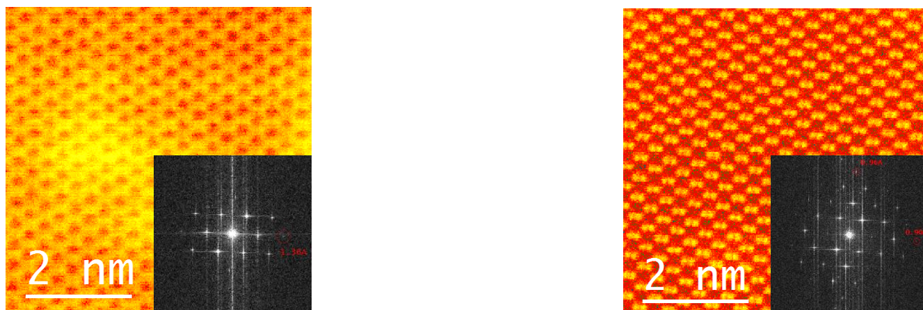
Figure 3. HR-STEM images of Si [110] with the monochromator excited ( dE=0.21\text{eV} ). Left: at 30kV, in the FT insert the 1.36Å reflection is visible. Right: at 80 kV; in the FT insert the 0.90Å reflection is visible
