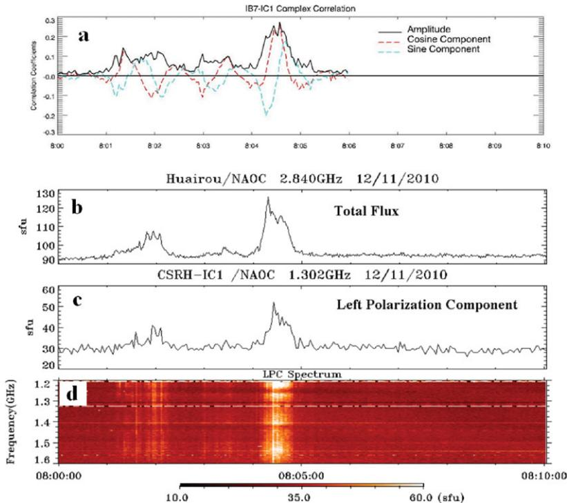
**Figure 1.** Panel a: Observed fringe included Cosine and Sine component with IB7-IC1 baseline. Panel b: Total flux profile observed by 2840M spectrometer in Huirou station. Panel c: Left polarization component profile observed by antenna IC1. Panel d: LPC spectrum observed by antenna IC1.
