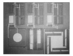
**ON THE COVER:** Ferroelectric thin films are being applied in a diverse range of applications, including microelectromechanical systems. Some examples are (from left to right) an acoustic sensor, a double supported microbeam accelerometer, and a tactile force sensor. For more information, see the section that begins on page 29.
