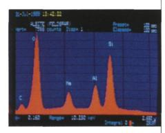
High sensitivity elemental analysis is possible with the addition of an EDS system.
