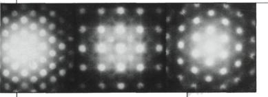
High resolution, electron microdiffraction analysis may require several tilt angles.
