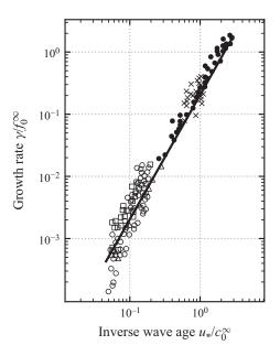
FIGURE 2. Non-dimensional, deep-water wave-energy growth rate  $\gamma/f_0^{\infty}$  versus inverse wave age,  $u_*/c_0^{\infty}$  with  $u_*$  the wind's friction velocity and  $c_0^{\infty} = \sqrt{g/k}$  the unforced, linear, deep-water phase speed. The filled symbols represent laboratory measurements while the hollow symbols represent field measurements (from Komen *et al.* 1994). The solid line represents the fit parameterized by Banner & Song (2002).
