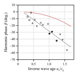
FIGURE 8. Harmonic phase  $\beta$  versus inverse wave age  $u_*/c_0$  (symbols) for the Leykin *et al.* (1995) laboratory experiments. The black, dashed line is the Leykin *et al.* (1995) linear fit. Theoretical HP  $\beta$  (solid red) are given for the generalized Miles pressure profile with  $\psi_P = 3\pi/4$ , kh = 2.5 and  $\varepsilon = 0.15$ , and conversion of  $u_*/c_0$  to  $Pk/(\rho_w g)$  is given by (5.6) (cf. § 5.3).
