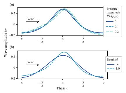
FIGURE 6. Wave profile  $k\eta$  versus phase  $\theta$  for  $\varepsilon = 0.2$ ,  $\psi_P = 3\pi/4$  and the generalized Miles pressure profile for (a) kh = 1.0 and variable  $Pk/(\rho_w g)$  (see legend) and (b)  $Pk/(\rho_w g) = 0.1$  and variable kh (see legend).
