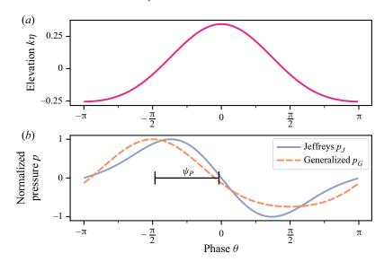
FIGURE 1. (a) Non-dimensional, right-propagating Stokes wave  $k\eta$  (2.18) as a function of phase  $\theta = kx - \omega t$  with  $\varepsilon = 0.2$ . (b) Normalized surface pressure profiles  $p(\theta)$  as described in (2.13) and (2.14); see legend. The maximum pressure magnitude is normalized to unity (arbitrary units), and a value of  $\psi_P = \pi/2$  was chosen to facilitate comparison with the Jeffreys profile with  $\psi_P$  positive corresponding to wind blowing to the right.
