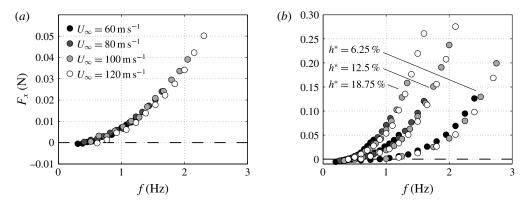
FIGURE 8. Dimensional thrust as a function of frequency at various free stream velocities for (a) pitching at  $\theta_0 = 7^{\circ}$  and (b) heaving at various  $h^* = h_0/c$ .
