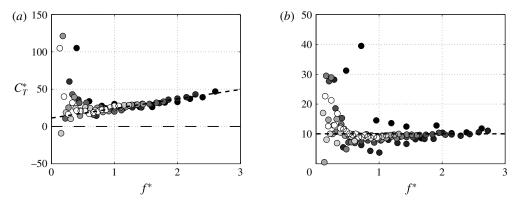
FIGURE 7. Newly non-dimensionalized thrust as a function of reduced frequency for (a) heaving and (b) pitching. Equations (6.2) and (6.3) are shown by the dashed lines. Colours are the same as in figures 3 and 5.
