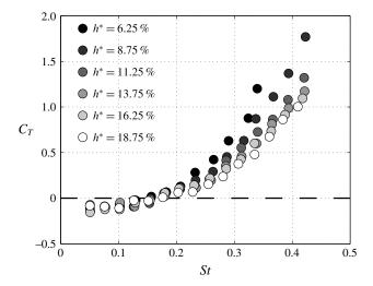
FIGURE 1. Time-averaged thrust coefficient  $C_T$  as a function of Strouhal number St for a heaving foil, for various heave amplitude to chord ratios,  $h^*$ . Experimental results from the current study. The parameters  $C_T$  and St are defined in § 2.
