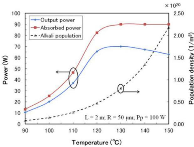
Figure 5. Absorbed power, output power, and population density ( $n_0$ ) versus temperature of Case 1.
