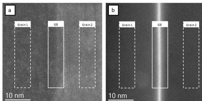
**Figure 2.** Figures 2a and 2b show the grain boundaries that exhibited minimal and strong segregation. Each image is a high-angle annular dark field image and the three boxes visualize the raster scan method.
