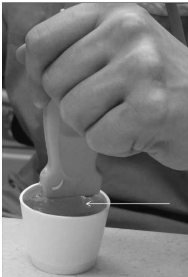
Figure 2: Ultrasound Technique with Model Secured in Gelatin Background. The anterior half of the gelatin globe is exposed from the gelatin background in the cup (arrow). It is then coated with ultrasound gel to enhance transmission. The probe is held at an angle perpendicular to the anterior exposed globe surface, directed straight at the 3D printed disc located on the posterior surface of the globe.
