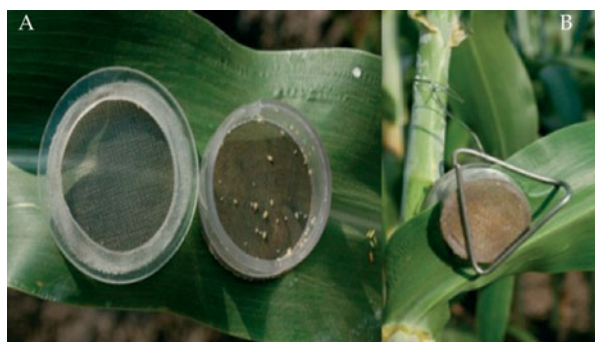
Plate 3. Clip cage used to confine the sugarcane aphid Melanaphis sacchari to the leaves of sorghum (a = aphids released inside the clip cage and b = clip cage placed on the sorghum leaf and tied with a galvanized iron wire around the stem).
