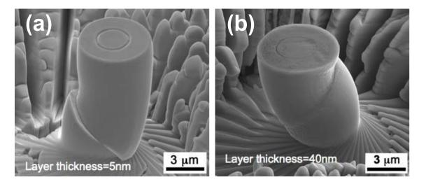
**Figure 3:** SEM micrographs of micropillars after compression. **(a) 5** nm Cu/Nb multilayer underwent 25% true strain before failing at the shear surface shown. **(b)** 40 nm multilayer deformed to 35% true compressive strain with failure in shear without fracture
