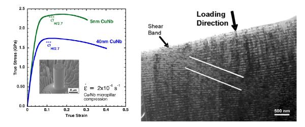
**Figure 1 (left):** Compression curves for 40 nm and 5 nm Cu/Nb multilayers. **Inset:** SEM micrograph of micropillar of 5 nm Cu/Nb multilayer in the as-prepared condition. Pillar height is 8 microns, and diameter is 4 microns. Layer interfaces are perpendicular to the long axis of the micropillar.
