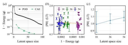
Figure 14. The 25th, 50th and 75th percentiles of (a) the reconstruction error of figure 4 from twenty different latent spaces of different size, (b) the PH as a function of the reconstruction error and (c) the medians of the PH of (b) as a function of the latent space size. The line in (b) is obtained by linear regression.
