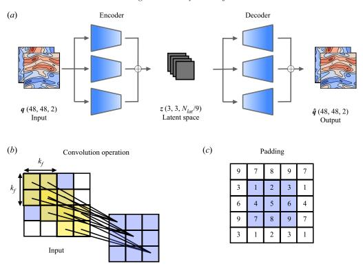
Figure 2. (a) Schematic representation of the multiscale autoencoder, (b) convolution operation for filter size  $(2 \times 2 \times 1)$ , stride = 1 and padding = 1 and (c) periodic padding. In (b,c), blue and white squares indicate the input and the padding, respectively. The numbers in (c) indicate pictorially the values of the flowfield, which can be interpreted as pixel values.
