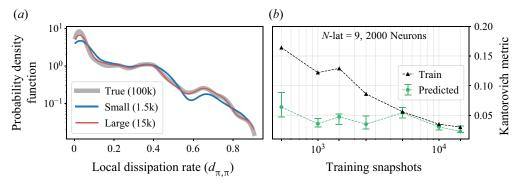
Figure 15. (a) P.d.f. of the local dissipation rate,  $d_{\pi,\pi}$ , in the training set for different numbers of training snapshots. (b) The 25th, 50th and 75th percentiles of the Kantorovich metric for the training set (Train) and for the CAE-ESN (Predicted) as a function of the training set size. Quasiperiodic regime.
