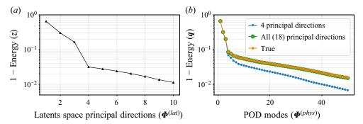
Figure 5. (a) Energy as a function of the latent space principal directions and (b) energy as a function of the POD modes in the physical space for the field reconstructed using 4 and 18 (all) latent space principal direction and data (True).
