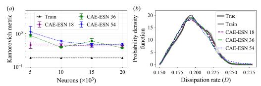
Figure 17. (a) The 25th, 50th and 75th percentiles of the Kantorovich metric of the dissipation rate, for the training set (Train) and for different reservoir and latent space sizes. (b) P.d.f. for the true and training data, and predicted by 10 000 neurons CAE-ESNs.
