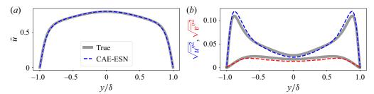
Figure 20. Profile of (a) mean streamwise and (b) fluctuating streamwise and wall-normal velocity profiles. Grey line: true statistics. Red/blue dashed lines: statistics from the CAE-ESN.
