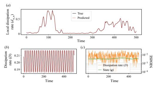
Figure 10. Prediction of (a) the local and (b) the average dissipation rate in the quasiperiodic case in the test set, i.e. unseen dynamics, for a CAE-ESN with a 2000 neurons reservoir and 9-dimensional latent space.
