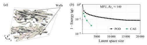
Figure 19. (a) Typical snapshot of the isosurfaces of the *Q*-criterion in the MFU. (b) Reconstruction error in the test set as a function of the latent space size for the MFU case.
