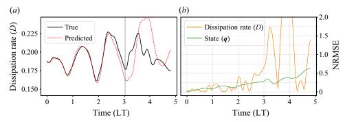
Figure 12. Prediction of the dissipation rate in the turbulent case in the test set, i.e. unseen dynamics, for a CAE-ESN with a 10 000 neurons reservoir and 36-dimensional latent space. The vertical line in panel (a) indicates the PH.
