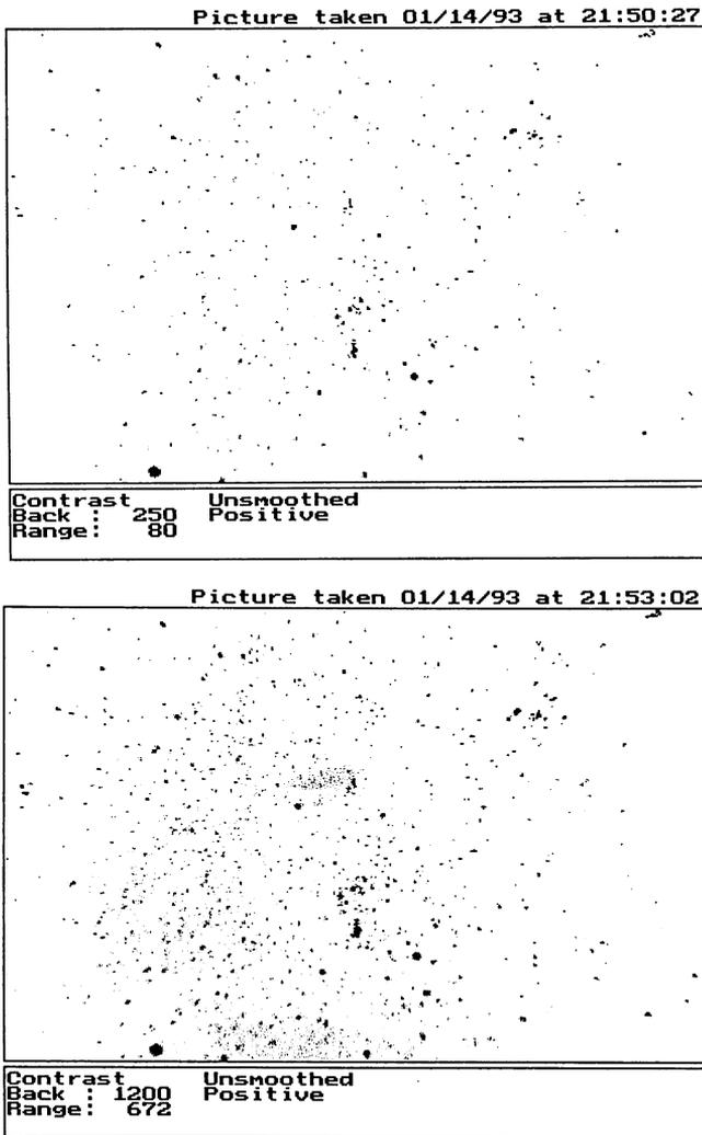
**Figure 2.** Test images of the Orion area obtained with slightly defocused 8.0 mm lens ( $f=8.0$  mm, 1:1.6) and SBIG ST-6 CCD camera. The field-of-view is roughly  $48 \times 40$  deg<sup>2</sup>. (a) Exposure 1 sec. (b) Exposure 9 sec.
