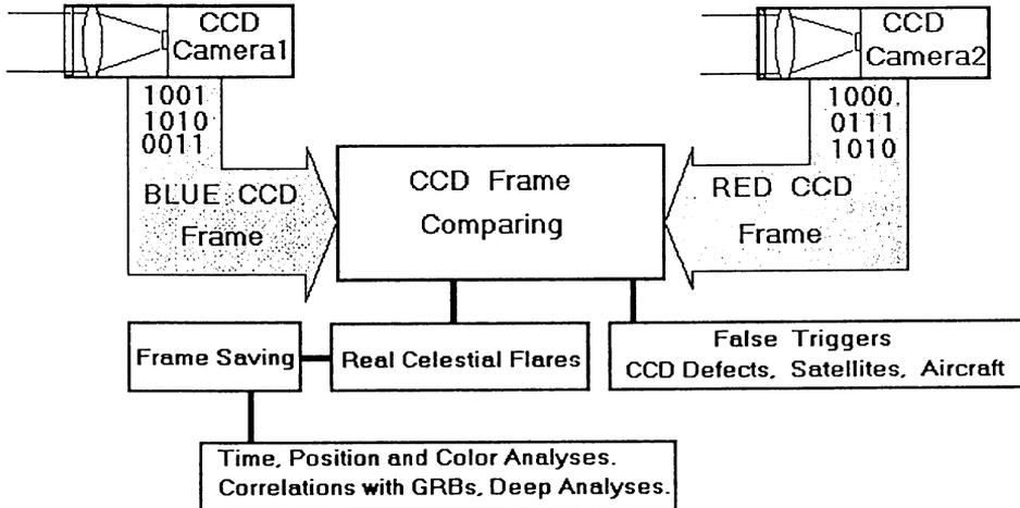
Figure 1. The proposed CCD monitoring configuration.
