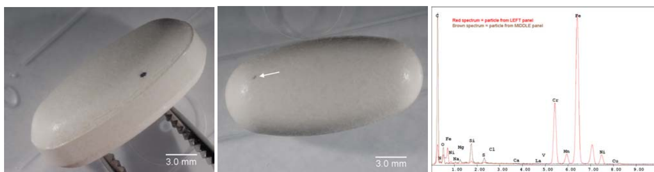
FIG. 1. Left, Middle: Tablets showing embedded particles; Right: EDS spectra of particles.
