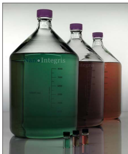
Figure 1. Metallic, unsorted, and semiconducting single-walled nanotubes (SWNTs) dispersed in a simple water-based solution.
