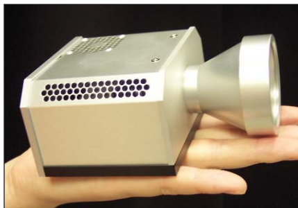
Figure 1. Superimaging's dual color automotive heads-up display (HUD) projector.
