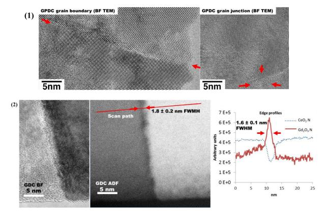
Fig. 1) Typical grain boundary [L] and junction [R] in GPDC shows structurally abrupt interfaces free of amorphous material. Data collected with JEOL-4000EX Fig. 2) Grain boundary in GDC imaged in BF TEM [L] and ADF STEM [M] with corresponding EELS line-scan profiles for Ce and Gd N-edges [R]. The indicated width in [R] corresponds to the FWHM of the Gd<sub>2</sub>O<sub>3</sub> EELS N-edge profile. Data collected with JEOL-4000EX, JEOL-2010F
