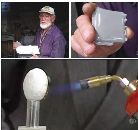
Top: Maurice Ward with his invention, Starlite. Bottom: Still image from 1990 episode of the BBC TV show Tomorrow's World , demonstrating Starlite's heat resistance and strength by wrapping it around an egg and blasting it with a Bunsen burner. Credits: BBC UK.
