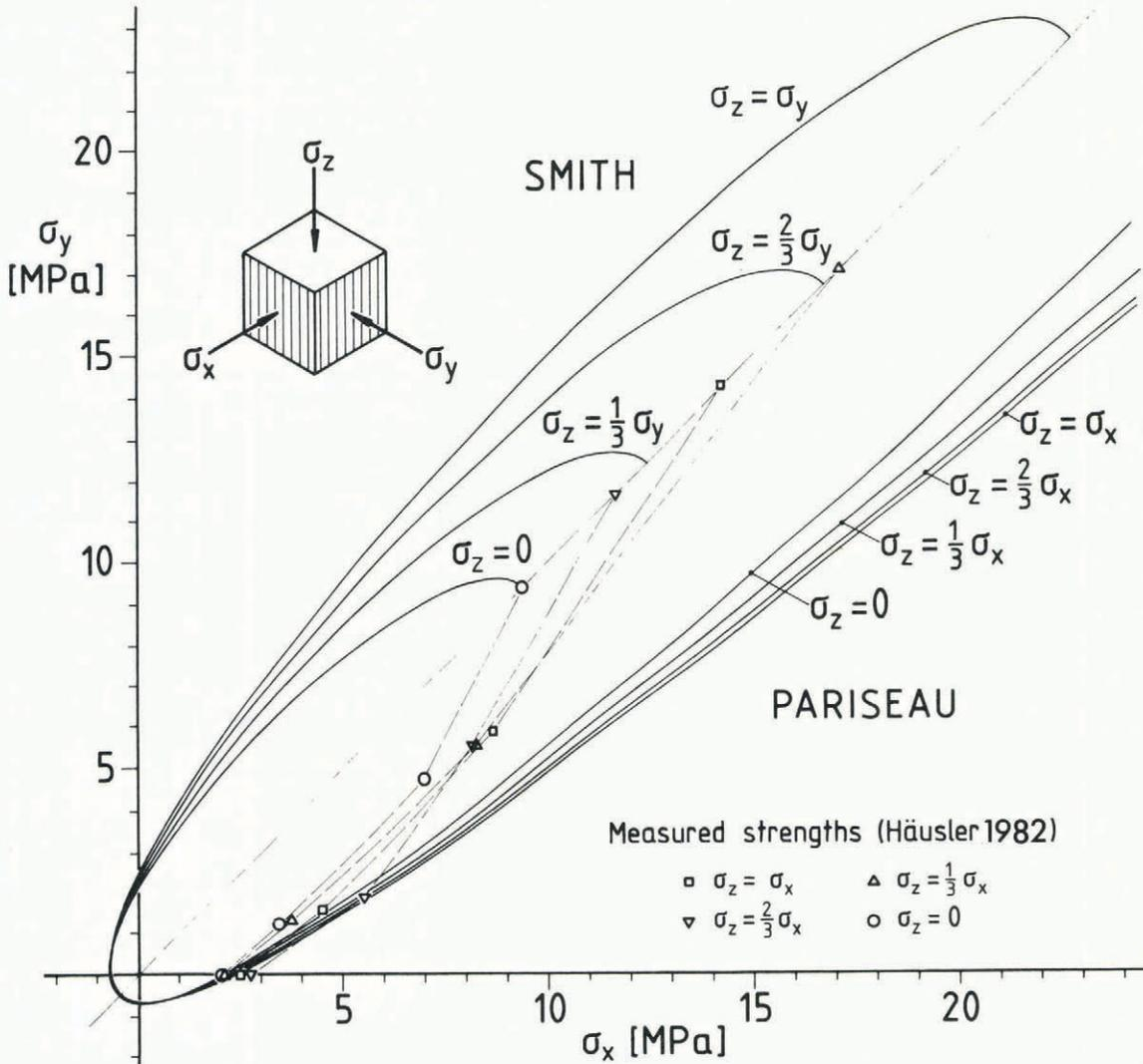
Fig.1. Projections of the Smith and Pariseau yield surfaces of saline ice ( $S = 10.6\%$  NaCl at the moment of sampling,  $T_I = -10^\circ\text{C}$ ,  $\dot{\epsilon} = 2.0 \times 10^{-4} \text{ s}^{-1}$ ) and of corresponding measured ice strengths onto the  $\sigma_x$ - $\sigma_y$ -plane of the principal stress space.
