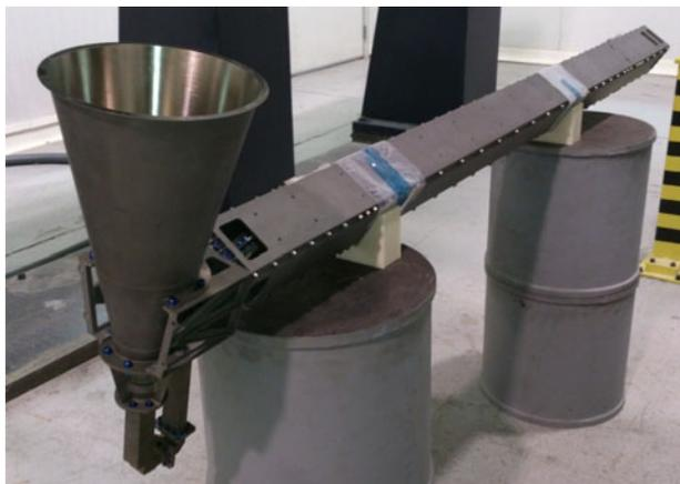
Fig. 2. RFA Engineering Qualification Model with structural boom.
