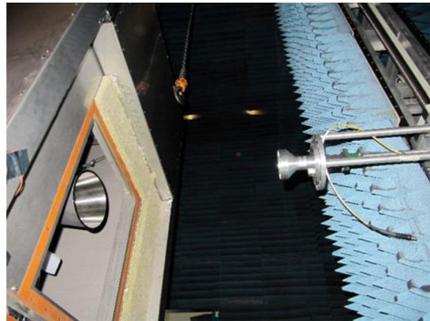
Fig. 6. Overview of RF oven placed in front of planar system.
