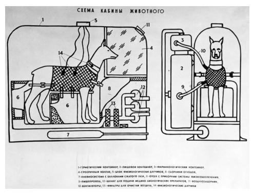
Figure 2. Schematic of the *Sputnik 2* cabin with dog technology. The dog's suit provided an interface with the life-support, monitoring and restraint systems in the cabin. Source: RGANTD fond 35, opis' 3, delo 57.
