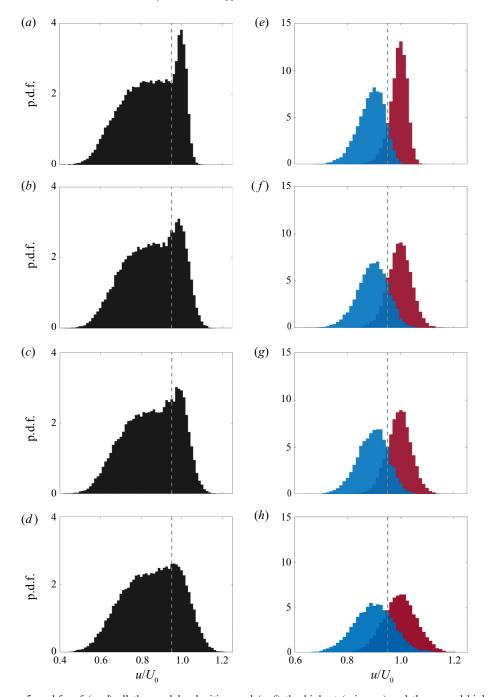
Figure 5. p.d.f.s of (a-d) all the modal velocities, and (e-f) the highest (crimson) and the second highest (blue) modal velocity, found in all PIV fields for cases REF, A, B and C, respectively, from top to bottom. The grey dashed lines mark  $u=0.95U_0$ .
