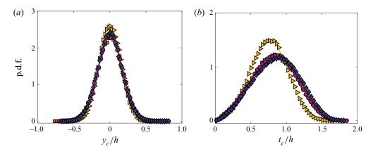
Figure 14. p.d.f. of (a) the core's centre location and (b) core thickness for cases REF ( $\triangleright$ , yellow), A ( $\blacksquare$ , orange), B ( $\bullet$ , purple) and C ( $\blacklozenge$ , navy blue).
