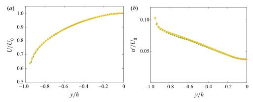
Figure 2. (a) Mean velocity, and (b) streamwise turbulence intensity profiles normalized by the centreline mean velocity for REF at X/H = 87 ( $\blacktriangleright$ , yellow), and X/H = 100 ( $\star$ , green).
