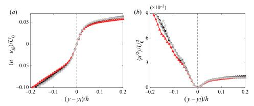
Figure 21. Profiles of streamwise (a) velocity, and (b) turbulent fluctuations, conditionally averaged across the core boundary for HMC fields identified by a presumed threshold value of  $1.035U_0$  ( $\bullet$ , black),  $1.065U_0$  ( $\blacktriangle$ , red),  $1.095U_0$  ( $\blacksquare$ , dark grey) and  $1.125U_0$  ( $\star$ , light grey). The dashed line indicates the core boundary.
