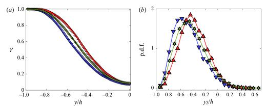
Figure 16. (a) Intermittency ( $\gamma$ ) profiles, and (b) p.d.f. of the core's lower boundary location for LMCs ( $\nabla$ , blue), OCs ( $\star$ , green) and HMCs ( $\triangle$ , red) of case C.
