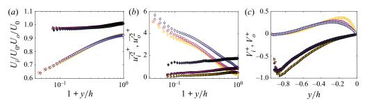
Figure 13. Weighted average profiles by  $\gamma$ , i.e. inside the core (symbols with black border), and by  $(1 - \gamma)$ , i.e. outside of the core (open symbols) of (a) mean streamwise velocity, (b) streamwise turbulent fluctuations and (c) mean vertical velocity for cases REF ( $\triangleright$ , yellow), A ( $\blacksquare$ , orange), B ( $\bullet$ , purple) and C ( $\blacklozenge$ , navy blue).
