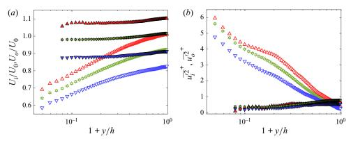
Figure 17. Weighted average profiles by  $\gamma$ , i.e. inside the core (symbols with black border), and by  $(1 - \gamma)$ , i.e. out of the core (open symbols) of (a) mean streamwise velocity, and (b) streamwise turbulent fluctuations for LMCs ( $\P$ , blue), OCs ( $\star$ , green) and HMCs ( $\P$ , red) of case C.
