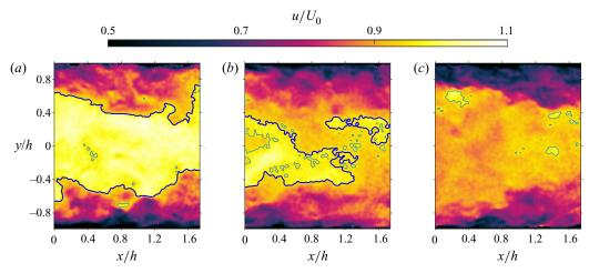
Figure 6. Sample instantaneous streamwise velocity fields for case C, showing (a) a continuous core, (b) a discontinuous core and (c) a 'No QC' example. Contour lines of  $u_{th} = 0.95U_0$  are indicated with blue lines. The thicker lines highlight the QC boundary.
