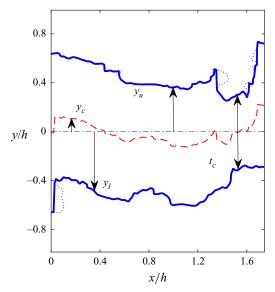
Figure 11. Enveloped (solid blue line) and un-enveloped (blue dotted line) core boundaries of the velocity field in figure 6(a). Core location and thickness parameters are depicted. The red dashed line indicates the core centre, i.e. midpoint between the upper and lower boundary. The grey dash-dot line shows the channel centreline.
