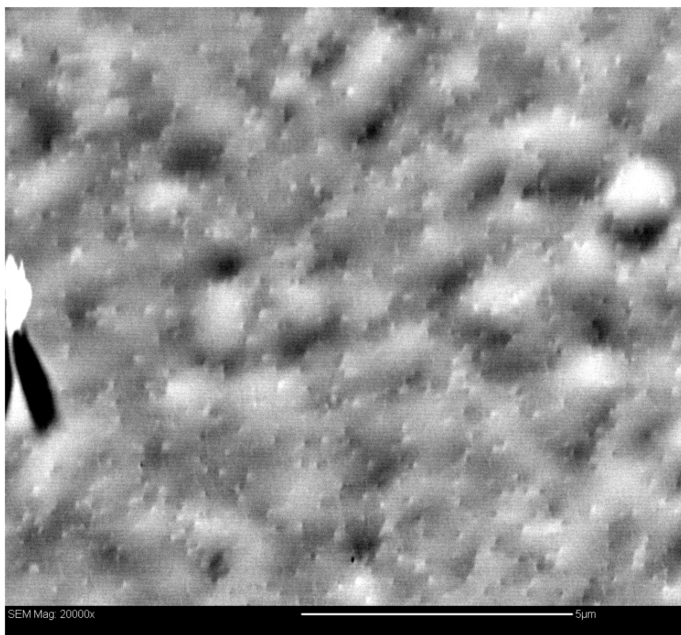
Figure 2. ECCI micrograph of a Ge film on Si. Threading dislocations manifest as bright dots in the image. (The bright feature on the left is surface debris and the adjacent dark contrast is an electron shadow it creates.)
