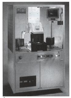
Optical Edge Bead Exposure System: Stand-alone Model 2000 from Optical Associates is designed to handle semiconductor wafers up to 8 in. (20.3 cm) in diameter. The system uses a shadow mask alignment module to facilitate setup of a mask to expose the edge and other areas requiring exposure during wafer processing. The system can use up to a 2000 W exposure tool, and throughput can be matched to user requirements.
