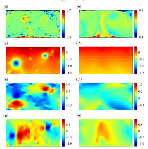
Figure 1. Snapshots of the (a,c,e,g) DNS  $(4096 \times 2048 \text{ grid})$  and (b,d,f,h) coarse no-model simulation  $(64 \times 32 \text{ grid})$  in statistically steady states. From panels (a,b) to (g,h), we show temperature, pressure, horizontal velocity and vertical velocity.
