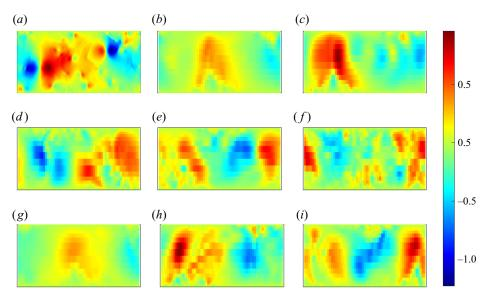
Figure 6. Vertical velocity fields in statistically steady states. Shown are the reference solution and the results obtained with coarse numerical simulations M0–7. The colour scheme is the same as used for the vertical velocity fields fields shown in figure 1. (a) DNS, (b) M0, (c) M1, (d) M2, (e) M3, (f) M4, (g) M5, (h) M6, (i) M7.
