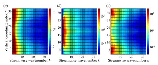
Figure 2. Correlation times  $\tau_{k,l}$  of the Fourier coefficients for the (a) horizontal velocity, (b) vertical velocity and (c) temperature measured from the high-fidelity data.
