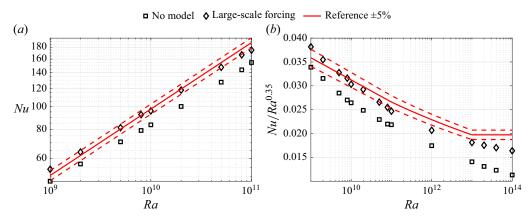
Figure 15. Measured Nusselt numbers as a function of the Rayleigh number. The solid red line shows reference Nusselt number predictions from the literature, with 5 % error margins given by the dashed lines. The no-model and large-scale forcing results are obtained with configurations M0 and M1, respectively. The reference scaling exponents are 0.285 for  $10^9 \le Ra \le 10^{13}$  and 0.35 for  $Ra \ge 10^{13}$ .
