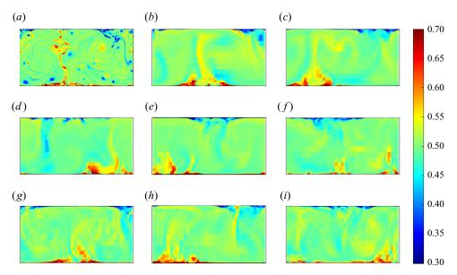
Figure 3. Temperature fields in statistically steady states. Shown are the reference solution and the results obtained with coarse numerical simulations M0–7. The colour scheme is the same as used for the temperature fields shown in figure 1. (a) DNS, (b) M0, (c) M1, (d) M2, (e) M3, (f) M4, (g) M5, (h) M6, (i) M7.
