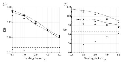
Figure 14. Comparison of the final rolling mean values of the (a) total kinetic energy (KE) and (b) Nusselt number for for different scalings of the correlation times  $\tau_{k,l}$  used in the model. The model results are displayed using the symbols in table 1.
