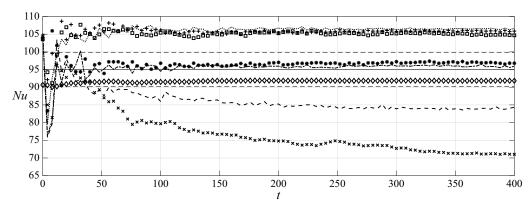
Figure 11. Comparison of the rolling mean of the Nusselt number over time. The solid line at Nu = 95 shows the theoretically predicted value, with 5% error margins given by the dashed lines. The model results are displayed using the symbols in table 1.
