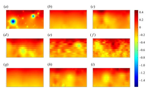
Figure 4. Pressure fields in statistically steady states. Shown are the reference solution and the results obtained with coarse numerical simulations M0–7. The colour scheme is the same as used for the pressure fields shown in figure 1. (a) DNS, (b) M0, (c) M1, (d) M2, (e) M3, (f) M4, (g) M5, (h) M6, (i) M7.
