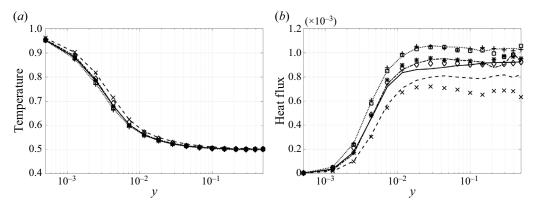
Figure 8. Comparison of the (a) time-averaged temperature and (b) time-averaged heat flux measured along horizontal cross-sections of the domain and displayed as a function of the wall-normal distance. The solid line shows the mean values of the filtered DNS, the model results are displayed using the symbols in table 1.
