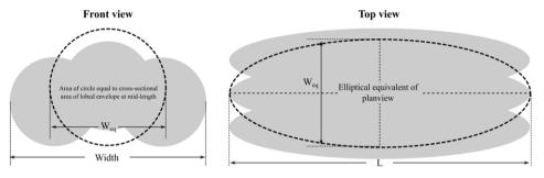
Figure 7. Equivalent ellipsoid (reproduced from Ref. (29)).
