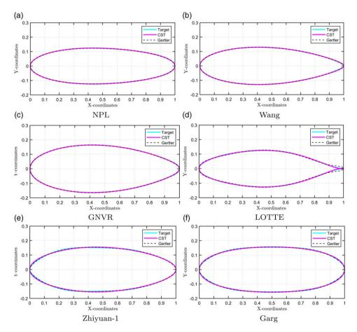
Figure 2. Standard envelope profile generated using CST and Gertler method.
