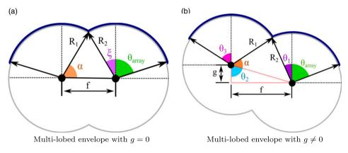
Figure 13. Geometry of the solar array.
