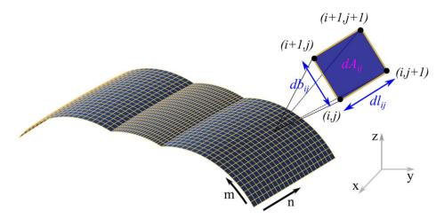
Figure 12. Schematic of solar array grid on the envelope.
