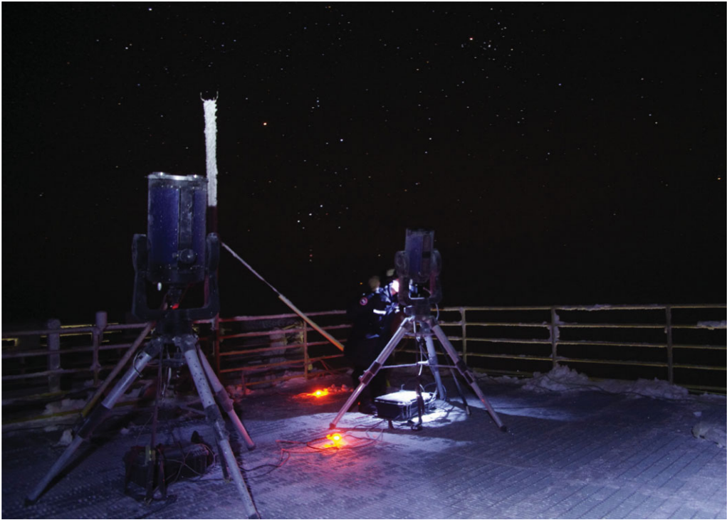
Figure 3. An observer checking on DIMM and MASS/DIMM site-testing telescopes deployed on the PEARL observing platform. Behind is the ice-covered mast of the meteorological station, beyond and to the right is the constellation Orion. Photo: Pierre Fogal.
