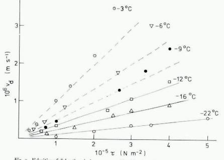
Fig. 2. Velocities of dislocations in ice as measured by Mai (1976) using X-ray topography.
