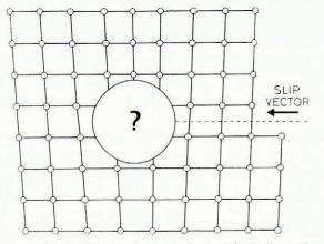
Fig. 1. An edge dislocation in a square lattice (after Read, 1953).
