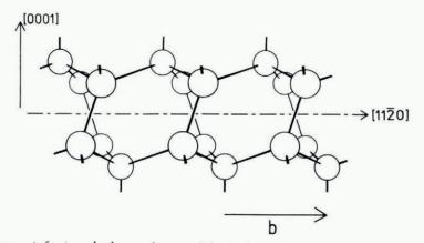
Fig. 6. The arrangement of water molecules around a screw dislocation lying along the [1120] axis indicated by the broken line.
