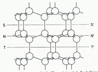
Fig. 4. The arrangement of molecules in the structure of ice Ih. The c-axis is vertical. Basal slip is normally assumed to occur on planes like ss' or TT'.
