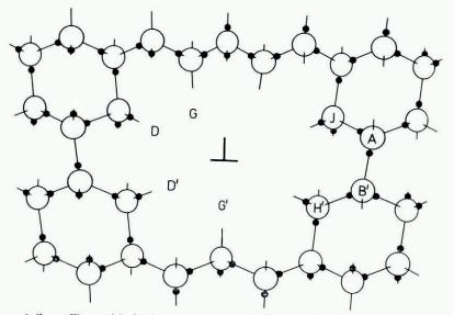
Fig. 8. Diagram similar to Figure 5(a) showing arrangement in (1700) plane of molecules around a 60° dislocation with a non-crystalline core incorporating 8 lattice sites. The disordered molecules in the core are not shown.
