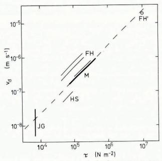
Fig. 3. Collected measurements of dislocation velocity  $v_{d}$  as function of stress  $\tau$  at temperatures of  $-15^{\circ}$  to  $-18^{\circ}C$ . M: Mai (1976), X-ray topography, -16°C. FH: Fukuda and Higashi (1973), X-ray topography, -18°C. JG: Jones and Gilra (1973), X-ray topography, -15°C, range of values at single stress. HS: Higashi and Sakai (1961), movement of tilt boundary as interpreted by Fukuda and Higashi (1973), -15°C.
