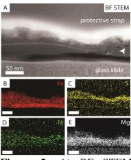
**Figure 2:** A) BF STEM image showing the complex stratigraphy of the melt and vapor deposit. The white arrow indicates the location of a nanophase Fe-Ni-S grain. EDS maps of the region showing the distribution of B) Fe, C) S, D) Ni, and E) Mg. 50 nm scale bars.
