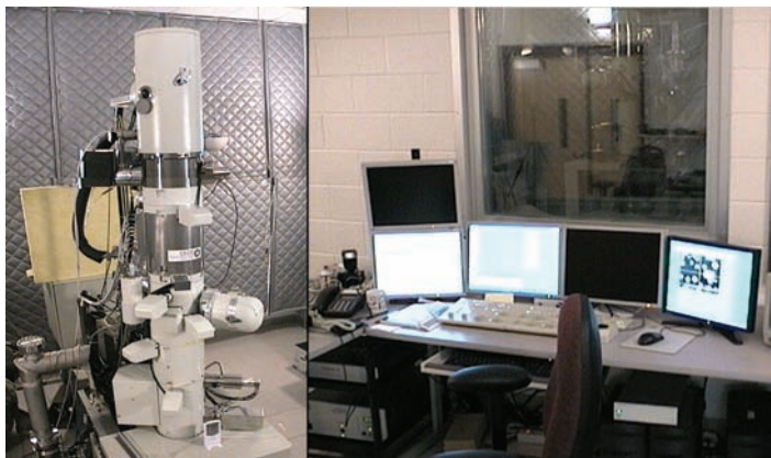
1: a) ORNL JEOL 2200FS at the HTML, b) the 'local' remote control of the instrument.
