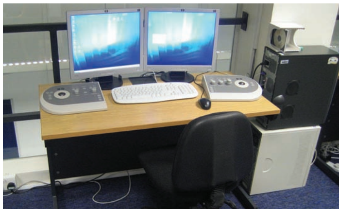
6: "Local" remote control of the Imperial College Titan. This workstation is connected to the microscope support PC via an optical fibre connection through to the microscope room.
