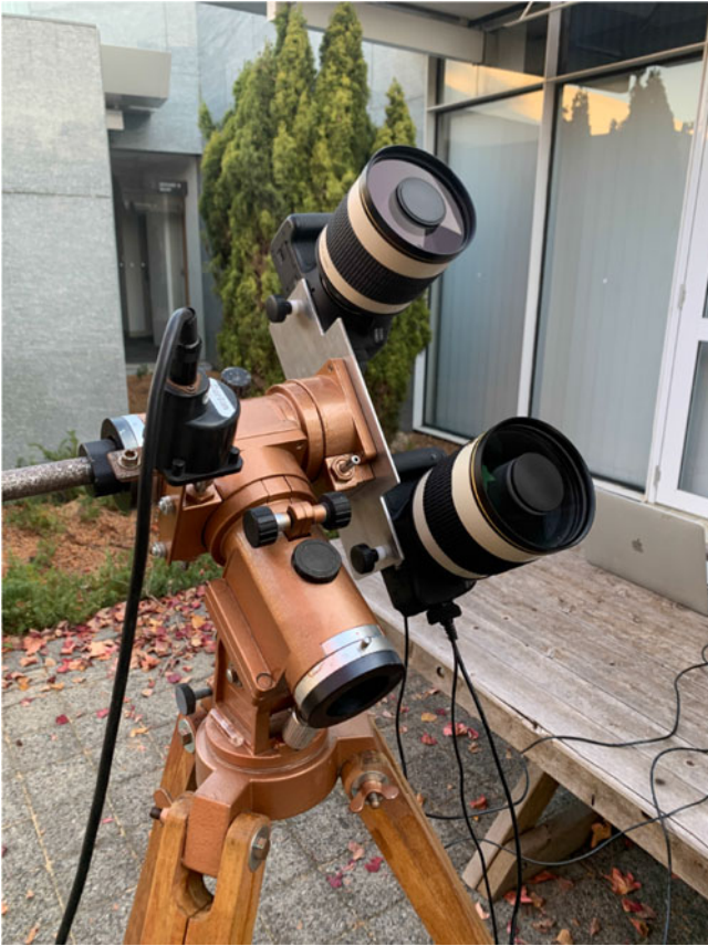
Figure 1. The two cameras mounted side-by-side for simultaneous operation. Camera A is at top, Camera B at bottom.
