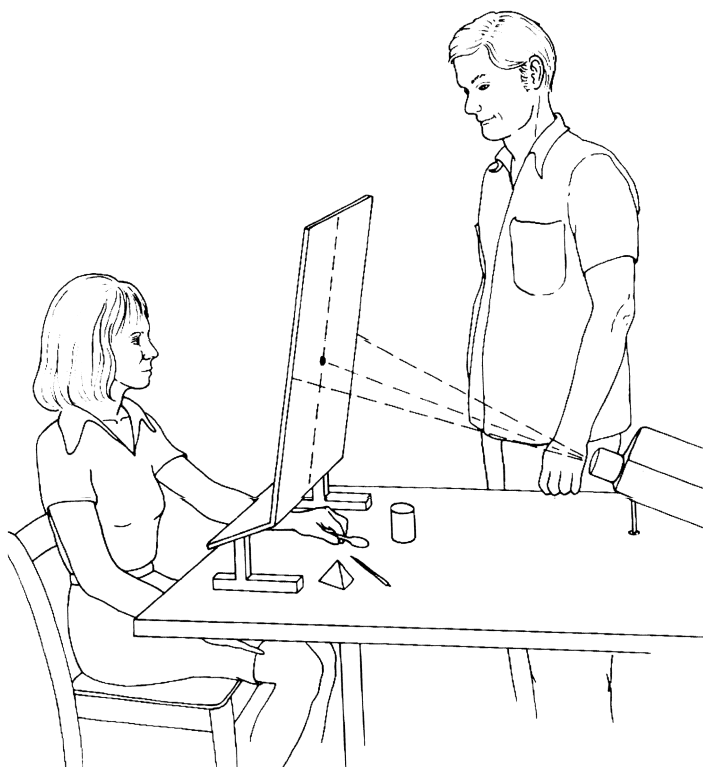
Figure 2. The experimental set-up used by Sperry (e.g. Ref. 4) The patient had a screen in front of the eyes onto which words would be shown, either to the left or right of a fixation cross in the middle of the screen. On the table below the screen, hidden from view, several objects were placed, some of which matched the words seen on the screen. See text for further explanation. Adapted from Ref. 2.
