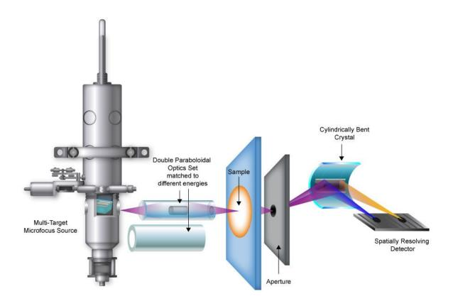
**Figure 1.** The x-ray absorption spectrometer design (XAS) comprises of innovations in the x-ray source and optic technology to enable high spectral and spatial resolutions at high throughput
