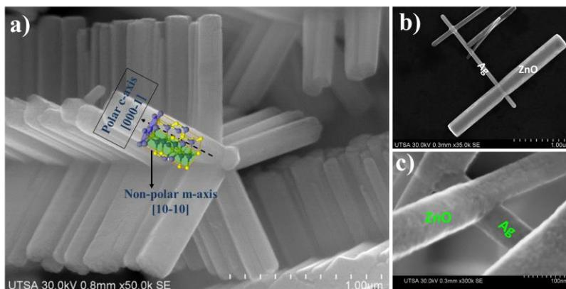
**Figure 1.** SEM image of a multi-pentagonal arrangement of Ag/ZnO nanorods. a) lateral-cross view section of an experimental nanostructure as growth by microwave irradiation process. b) Controlling the time growing it is possible to obtain an Ag/ZnO nanostructure with ZnO nanorods partially distributed along the silver nanowire. c) ZnO nanorods growing on the pentagonal faces of silver nanowire.
