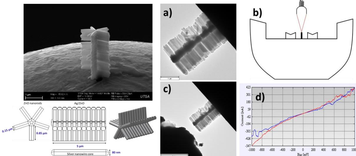
**Figure 2.** Single multi-pentagonal arrangement of Ag/ZnO. Left) view section of an experimental nanoantenna prepared in Focus Ion Beam (FIB) instrument. Once the Ag/ZnO is set up in a FIB grid *in-situ* TEM electrical measurements were performed. a) – c) shown a TEM image before the electrical probe reached the Ag/ZnO nanosystem closing the circuit. d) shows an  $I$  vs  $V$  experimental curve depicting a non-ohmic system as expected for the metal-semiconductor arrangement.
