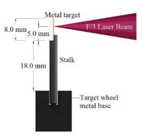
Figure 1. Schematic of target design and experimental arrangement.
