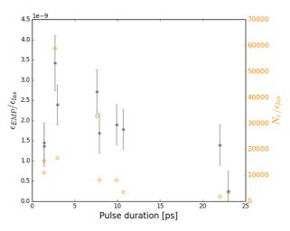
**Figure 3.** Plot of EMP energy and total number of escaping electrons versus laser pulse duration. The grey diamonds represent the ratio of EMP energy to on-target laser energy, while the orange diamonds represent the ratio of total electron number  $(N_e)$  to on-target laser energy. EMP data was taken from the B-dot West probe.
