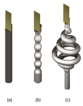
**Figure 8.** The three different stalk designs: (a) standard cylindrical geometry with a geodesic path length of 20 mm; (b) a sinusoidally modulated stalk with the same maximum cross-section as the standard cylinder and a path length of 30 mm; (c) spiral stalk design with an identical diameter to (a), but a geodesic path length of 115 mm.
