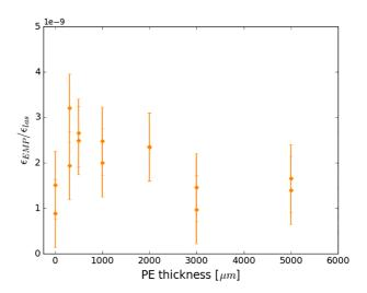
**Figure 13.** The ratio of EMP energy to laser energy versus thickness of PE backing on 1  $\mu$ m Cu targets as measured by the B-dot West probe.
