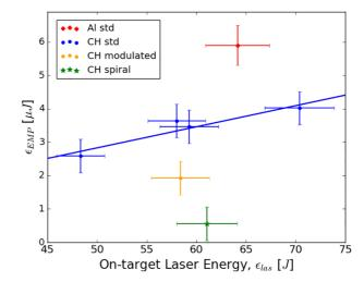
**Figure 7.** EMP energy versus on-target laser energy for a variety of different stalk designs (B-dot probe East). Laser focal intensity is between  $8 \times 10^{17} \ \mathrm{W \cdot cm^{-2}}$  and  $2 \times 10^{19} \ \mathrm{W \cdot cm^{-2}}$  for these shots. Also included is a linear fit to the standard CH cylindrical stalk data, as detailed in Figure 2.
