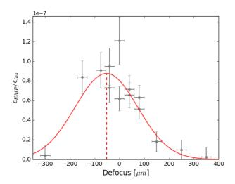
**Figure 5.** The ratio of EMP energy to laser energy plotted against defocus (as measured by the D-dot East probe). The Gaussian fit is meant as a visual aid, with a laser focal intensity of approximately  $1 \times 10^{18}~{\rm W\cdot cm^{-2}}$  at the Gaussian peak.
