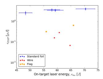
**Figure 6.** EMP energy as a function of on-target laser energy for wire, flag and standard foil designs (B-dot probe East). Laser focal intensity ranges from  $8 \times 10^{17} \text{ W} \cdot \text{cm}^{-2}$  to  $2 \times 10^{19} \text{ W} \cdot \text{cm}^{-2}$  on these shots and we have chosen a logarithmic *y*-axis to emphasize the drop in EMP. Notice how changing the wire diameter has led to a deviation from the linear relationship between EMP and on-target laser energy.
