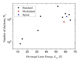
**Figure 9.** Total number of electrons recorded by the electron spectrometer as a function of on-target laser energy. Uncertainties in on-target laser energy are  $\sim 10\%$ .
