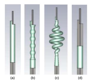
**Figure 11.** Side elevation of stalk designs used in 3D PIC simulations. Transparent grey sections represent a perfect electrical conductor (PEC), while the grey-green regions represent Teflon plastic. (a) Standard cylindrical stalk configuration: pure Teflon and PEC models were used. (b) Sinusoidally modulated Teflon stalk. (c) Teflon spiral stalk. (d) Half-length Teflon and PEC stalk.
