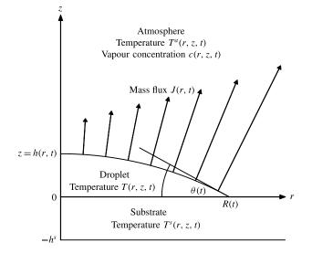
FIGURE 1. The geometry of a evaporating thin sessile droplet on a thin substrate.
