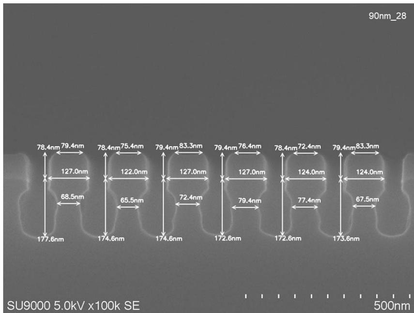
**Figure 2.** Result of extraction step for L/S hp = 90 nm.
