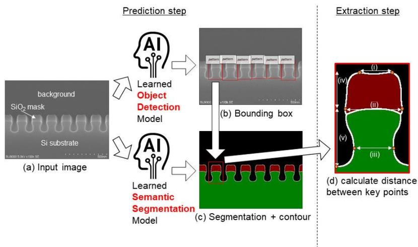
**Figure 1.** Flow of prediction and extraction steps of automated measurement tool.
