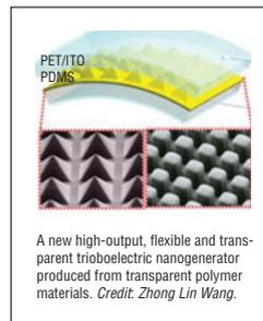
A new high-output, flexible and transparent triboelectric nanogenerator produced from transparent polymer materials. Credit: Zhong Lin Wang.
