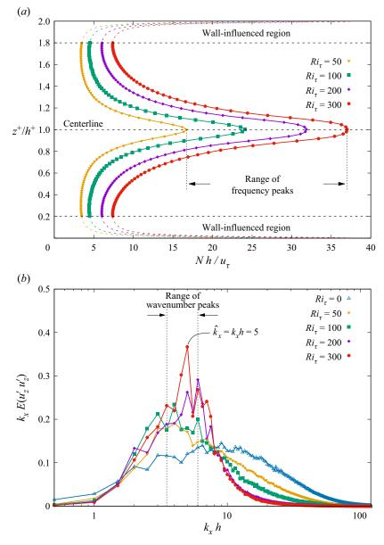
Figure 10. (a) Wall-normal behaviour of the mean Brunt-Väisälä frequency N for the different cases of stratified turbulence ( $Ri_{\tau} = 50$ ,  $Ri_{\tau} = 100$ ,  $Ri_{\tau} = 200$  and  $Ri_{\tau} = 300$ ). (b) Time-averaged premultiplied streamwise energy spectra of wall-normal velocity fluctuations  $k_x E(u'_z u'_z)$  evaluated on a wall-parallel (x-y) plane located at the channel centre.
