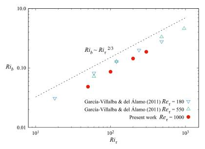
Figure 12. Bulk Richardson number,  $Ri_b$ , as a function of the shear Richardson number,  $Ri_\tau$ , for the present simulations at  $Re_\tau=1000$ , and for previous simulations at  $Re_\tau=180$  and  $Re_\tau=550$  (García-Villalba & del Álamo 2011). The proposed scaling  $Re_b\sim Ri_\tau^{2/3}$  is also explicitly indicated.
