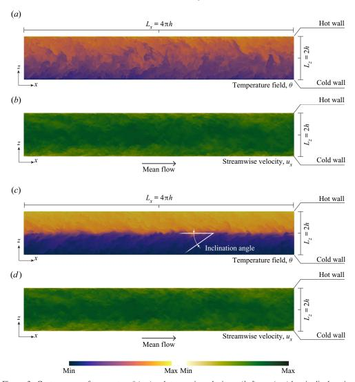
Figure 3. Contour maps of temperature  $\theta$  (a,c) and streamwise velocity  $u_x$  (b,d) on a (x-z) longitudinal section located at  $y = L_y/2$ . (a,b) Refer to the neutrally buoyant case,  $Ri_\tau = 0$  and (c,d) refer to the stably stratified case at  $Ri_\tau = 300$ . The temperature tilting induced by the vertical shear at the channel centre is also explicitly indicated (c).
