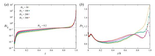
Figure 11. Wall-normal behaviour of the gradient Richardson number  $Ri_g$  (a) and of the turbulent Prandtl number  $Pr_t$  (b) for the different values of  $Ri_{\tau}$ . The threshold value  $Ri_g = 0.2$  is also explicitly shown in panel (a) (dashed line).
