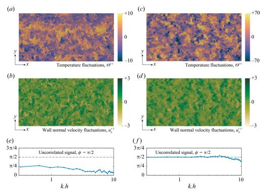
Figure 8. Temperature and velocity fluctuations on a wall-parallel (x-y) plane located at the channel centre for  $Ri_{\tau} = 0$  (a,b) and for  $Ri_{\tau} = 300$  (c,d). Phase of the cross-spectrum,  $\phi(C_{u_{\tau}^{\prime +},\Theta'^{\prime +}})$ , as a function of the wavenumber  $\kappa_w = kh$  for  $Ri_{\tau} = 0$  (e) and for  $Ri_{\tau} = 300$  (f).
