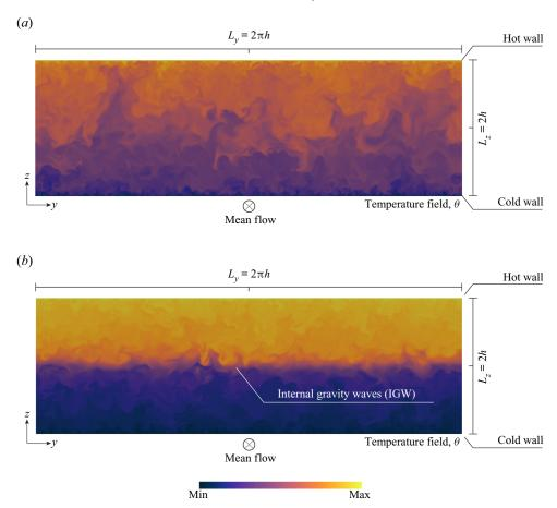
Figure 2. Contour maps of temperature,  $\theta$ , on a (y-z) cross-section located at  $x = L_x/2$ . (a) Refers to the neutrally buoyant case,  $Ri_\tau = 0$  and (b) refers to the stably stratified case at  $Ri_\tau = 300$ .
