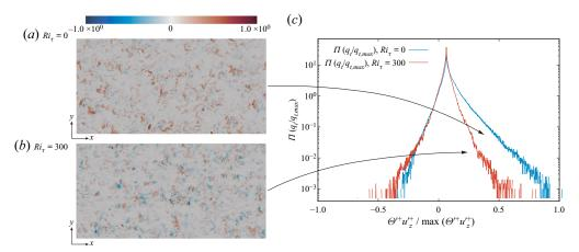
Figure 9. Contour map of the turbulent heat flux  $q_t = \langle \Theta^+ u_z^{\prime +} \rangle$  on a wall-parallel (x-y) plane located at the channel centre for  $Ri_{\tau} = 0$  (a), for  $Ri_{\tau} = 300$  (b) and corresponding probability density function  $\Pi(q_t/q_{t,max})$  (c).
