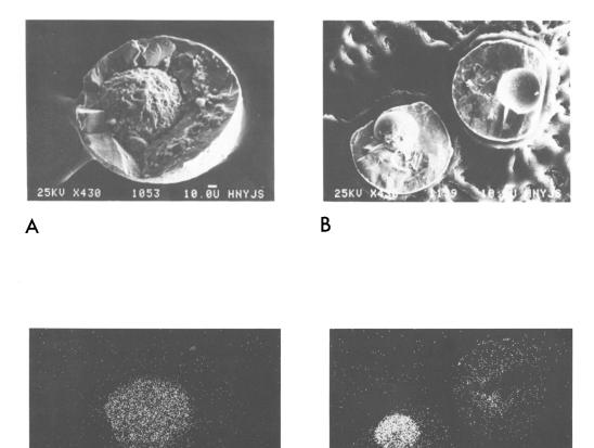
Figure 1. SEM Photographs of the iron spherules. A and B are broken iron spherules with the Ni-Fe core; C and D are respectively NiKa plane distribution pictures of A and B.
