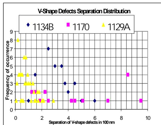
**Fig.7:** Frequency of the observation of the V-shaped defect as a function of the separation between two consecutive V defects is the highest for a doped sample with highest Al content and the lowest for the undoped lower Al content sample.
