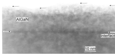
**Fig. 6:** High resolution TEM image of a doped 45% AlGaN layer on  $\sim 2 \mu\text{m}$  GaN on a sapphire substrate (sample **1129A**). Careful analysis of the growth front between V-shaped defects indicates 3D growth.
