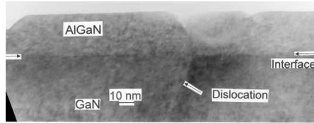
**Fig. 2:** High resolution image of an undoped AlGaN layer (sample 1170) layer on ~1.7-2.0  $\mu\text{m}$  GaN on a sapphire substrate showing V-shaped defects. Note that the growth between V-shaped defects is planar (2D). The V-shaped defect to the left initiated about 200 nm away from the AlGaN /GaN interface.
