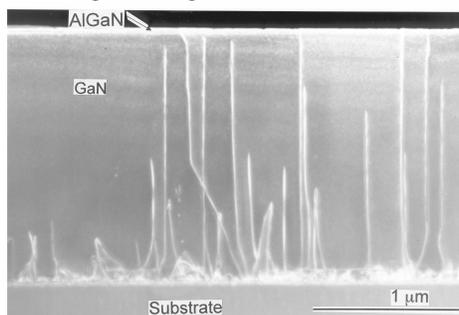
**Fig. 1:** Weak beam  $g=[0002]$  image of an undoped 30% AlGa<sub>x</sub>N layer (sample **1170**) layer on about 1.7-2  $\mu$  GaN layer on a sapphire substrate. Note presence of V-shaped defects. In many cases these defects appear to be associated with the threading dislocations.
