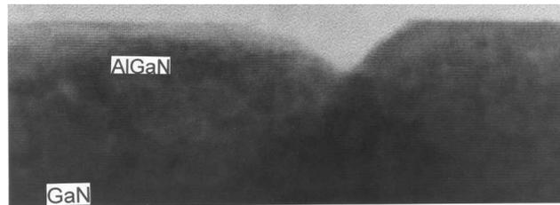
**Fig. 4:** High resolution TEM image of the cross-section of a doped 30% AlGaN layer on ~2  $\mu\text{m}$  GaN on a sapphire substrate (sample 1134B).
