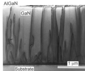
**Fig. 3:** TEM bright field image of the cross-section of a doped 30% AlGaN layer on ~2  $\mu\text{m}$  GaN on a sapphire substrate (sample 1134B).
