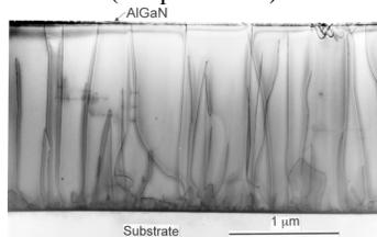
**Fig.5:** Bright field TEM image of the cross-section of a doped 45% AlGaN layer on ~2  $\mu\text{m}$  GaN on a sapphire substrate (sample 1129A).
