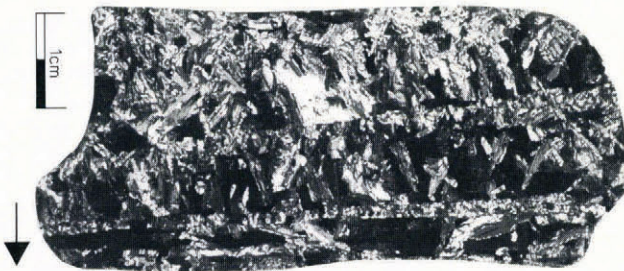
Fig. 3. Vertical thin-section photograph of a single pancake-ice disc as seen between crossed polarizers; here, as in the following photographs, the scale is in centimeters; the arrow points towards the bottom of the sampled floe.
