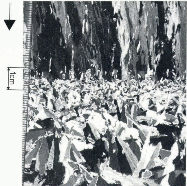
Fig. 6. Vertical thin-section photograph showing the lower part of an ice core taken on a floe, which was previously underlain by a layer of ice platelets; the irregular texture in the bottom half of the image represents a consolidated part of this layer, which we call "platelet ice".
