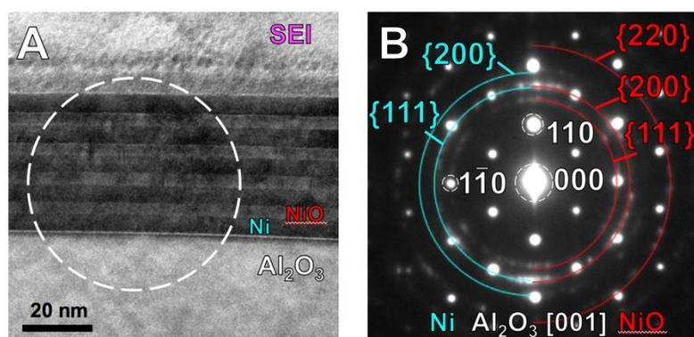
**Figure 1.** (A) HRTEM image of lithiated multilayer film with 5 bilayers of 5 nm Ni and 5 nm NiO on  $\text{Al}_2\text{O}_3$  substrate. Only the top NiO layer has undergone lithiation as substantial Li transport did not occur through the 5 nm thick Ni layer. (B) SAED from area indicated by dashed circle in (A). NiO diffraction rings are clearly seen, indicating the absence of any NiO conversion reaction to Ni in the lower layers of the structure.
