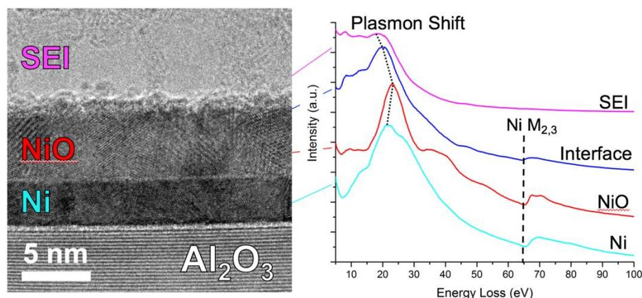
**Figure 2.** HRTEM image of Ni/NiO Bilayer Film on  $\text{Al}_2\text{O}_3$  substrate, with EELS spectra collected in different regions of the bilayer architecture. A Ni-containing interface has formed on top of the NiO layer, revealing part of the reaction mechanism during the early stages of conversion.
