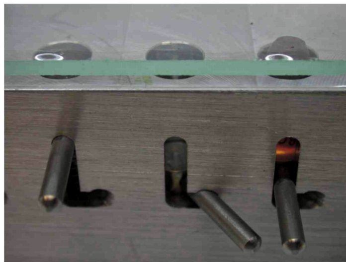
Figure 1. Close up view of aluminum apparatus for holding epoxy blocks against an acetate film under a glass plate. The spring-loaded lever can be retracted for block loading and released after the film and plate are clamped into place.
