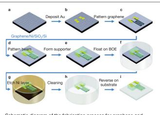
Schematic diagram of the fabrication process for graphene and epoxy hybrid cantilever system. Reproduced with permission from *Nano Lett.* (DOI: 10.1021/nl103618e). © 2011 American Chemical Society.
