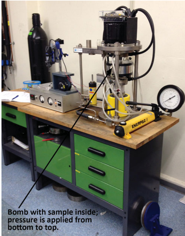
Fig. 6. The quick-press piston-cylinder (Depth of the Earth Department type) at the HPT laboratories of VU University Amsterdam. For calibration and set-up see, for example, Rai et al. (2013).
