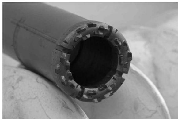
**Fig. 5.** Temperature-stabilized diamond rock-coring bit.
