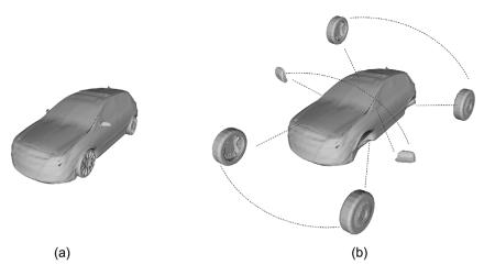
**Figure 1.** Comparison between a monolithic shape (a) and a structure-aware shape (b), where dash lines indicate structural interdependencies (i.e. support and symmetry) between components.
