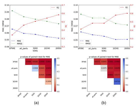
**Figure 8.** The comparison of prediction accuracy for the test set data of aircraft models using different VDRs with drag coefficients with three evaluation metrics: MAE ( $\downarrow$ ), RMSE ( $\downarrow$ ) and the  $R^2$  ( $\downarrow$ ) using (a) Auto-sklearn or (b) AutoGluon. The p-values resulting from the paired t-test for AE values are used to show the statistical difference.
