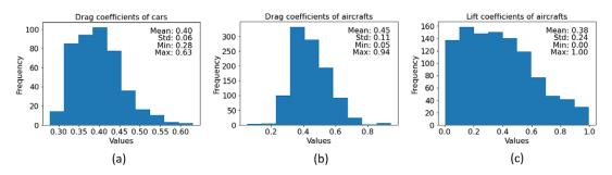
**Figure 4.** Histograms of (a) drag coefficients of car models, (b) drag coefficients of aircraft models and (c) lift coefficients of aircraft models with the mean, std, min and max values.
