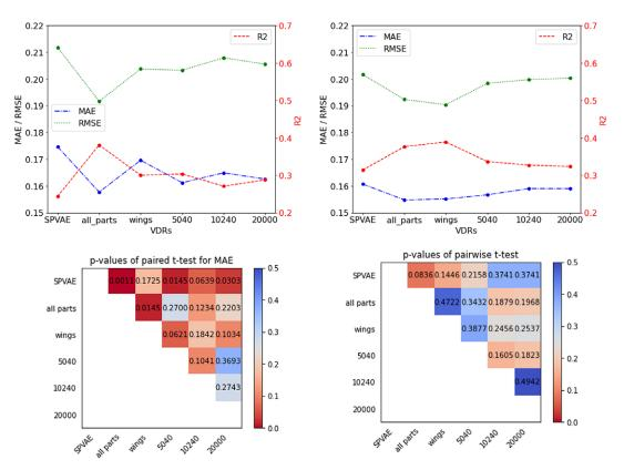
**Figure 9.** The comparison of prediction accuracy for the test set data of aircraft models using different VDRs with lift coefficients with three evaluation metrics: MAE ( $\downarrow$ ), RMSE ( $\downarrow$ ) and the  $R^2$  ( $\downarrow$ ) using (a) Auto-sklearn or (b) AutoGluon. The p-values resulting from the paired t-test for AE values are used to show the statistical difference.
