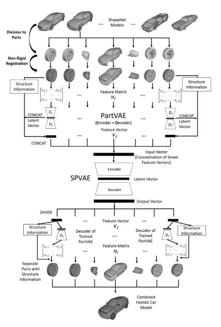
**Figure 3.** Overview of the data-driven structure-aware generative design module demonstrated using a car design case. The design module is implemented using SDM-NET (Gao *et al.* 2019*b*) that consists of PartVAEs and SPVAE.
