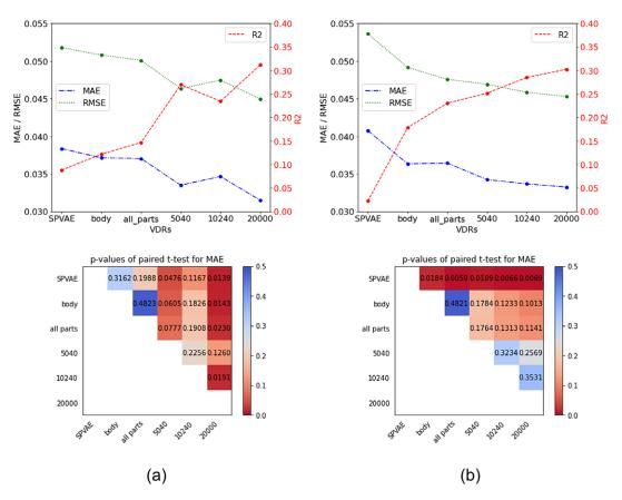
**Figure 7.** The comparison of prediction accuracy for the test set data of car models using different VDRs with drag coefficients with three evaluation metrics: MAE ( $\downarrow$ ), RMSE ( $\downarrow$ ) and the  $R^2$  ( $\downarrow$ ) using (a) Auto-sklearn or (b) AutoGluon. The p-values resulting from the paired t-test for AE values are used to show the statistical difference.
