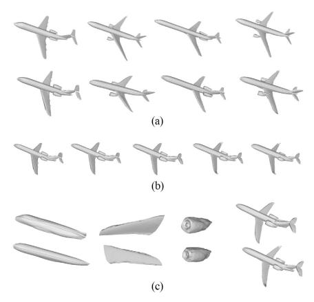
**Figure 6.** Examples of the generated shapes for aircraft models. (a) Reconstruction of aircraft models. (b) Shape interpolation of merged aircraft models. (c) Random generation of separate parts (fuselage, wings and engines) and merged aircraft models.
