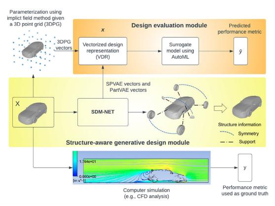
**Figure 2.** Overview of the research approach consisting of two key modules: the structure-aware generative design module and the design evaluation module
